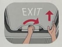
To open a rooftop exit, pull the handle, rotate, and push the hatch up.
